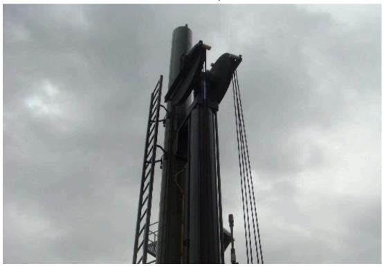
A Major International Oil Company in North Dakota recently installed an SSi Model 600 (containing a 125 Horse Power Control Unit), on an already existing well, where a conventional Beam Pump was producing approximately 40 barrels per day
