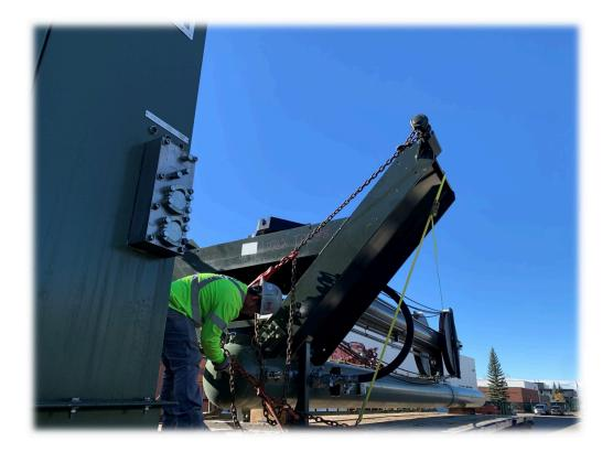
These units are operating at 5 strokes per minute and producing between 2,500 and 3,300 BBIs. per day but the Beam Pumps adjacent to these units are operating at 9 or 10 strokes per minute. On the assumption that the rods and downhole equipment will fail at the same number of cycles, the SSi Units operating at approximately half the speed for similar production, infers the time between well intervention is double allowing <u>further substantial cost savings</u>.
