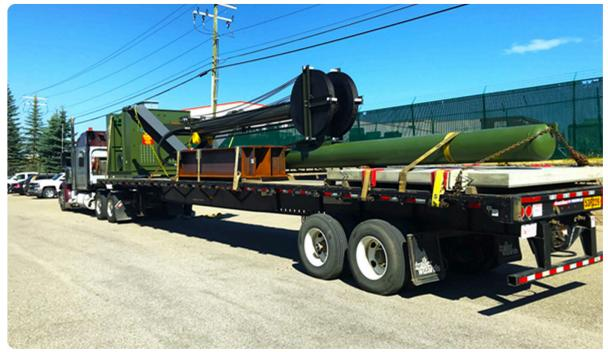
When comparing actual costs for Artificial Lift Equipment, it is very common to focus on the capital costs or initial cost to acquire the equipment, but the real costs that needs to be measured is the full scope of supply, cost of transportation, the installation costs which include the Piles, Concrete Bases as well as the cranes and auxiliary equipment required for an installation and the Through Life Cost.
