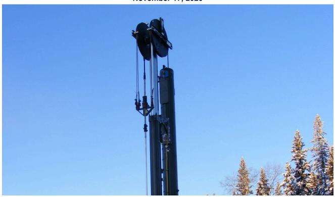
A Major Oil Producer in Northern Alberta has reported great success with their 210-inch stroke length, **SSi Model 250** (60 horsepower). The unit was installed nearly 10 years ago in Northern Alberta and has been running without any failure for all its 9 years, or 3,576 days of ongoing uninterrupted operation.
