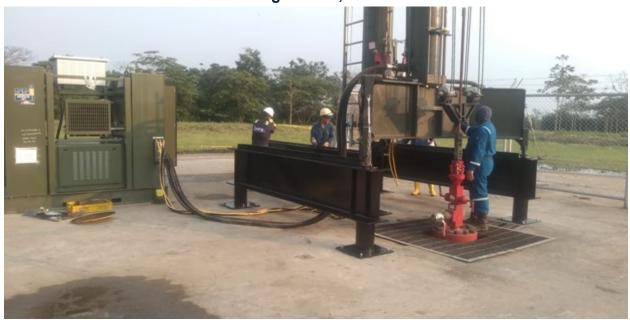
SSi Lift was approached by a Major Oil Company about providing Long Stroke Rod Lift Technology in one of their extra-heavy oil fields. This field had unsuccessfully tried using an ESP to produce but recorded higher costs due to premature failures after three months.
